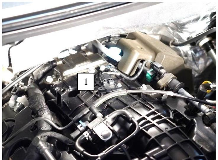
2. Install the supplied 1/8" NPT nipple on the MAP adapter. Blank off the second port on the MAP adapter if it is not in use. **Use thread sealant. Route the vacuum hose from the nipple towards your accessory. Use one of the supplied spring clamps to secure the vacuum hose onto the nipple.**
