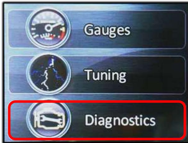
**Step 2** - In the “Diagnostics” menu, select “Settings,” then select “Device Info.” A screen will display with the nGauge Serial #, Voltage, BIOS, Firmware and Board. The important number to check is the “Firmware” number.
