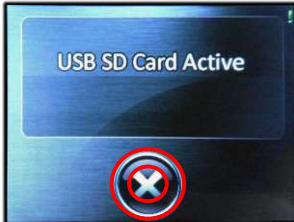
**Step 7** – Select “Diagnostics” from the main menu again, then select “Settings.” Use the down arrow til you see “Update from SD”, then select it. The device will find the firmware you put on the nGauge, then confirm you want to update it. Make sure the device does not get unplugged. The update should take 5-10 seconds to complete. The device will confirm the update is complete, then restart.
